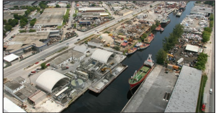
This aerial photo of the processing site shows the covered stockpiling areas and a barge being unloaded. The ship moored on the opposite bank illustrates the confined working space of the project.
